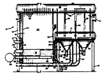
A fluidized bed boiler having a water-wall type construction has a steam-water natural circulation system for heat exchange. Vertical in-bed heat exchange tubes are provided and the steam drum of the boiler extends across the full length of the boiler combustion chamber and the convection heat exchange chamber. An air distributor grate is provided for introduction of
